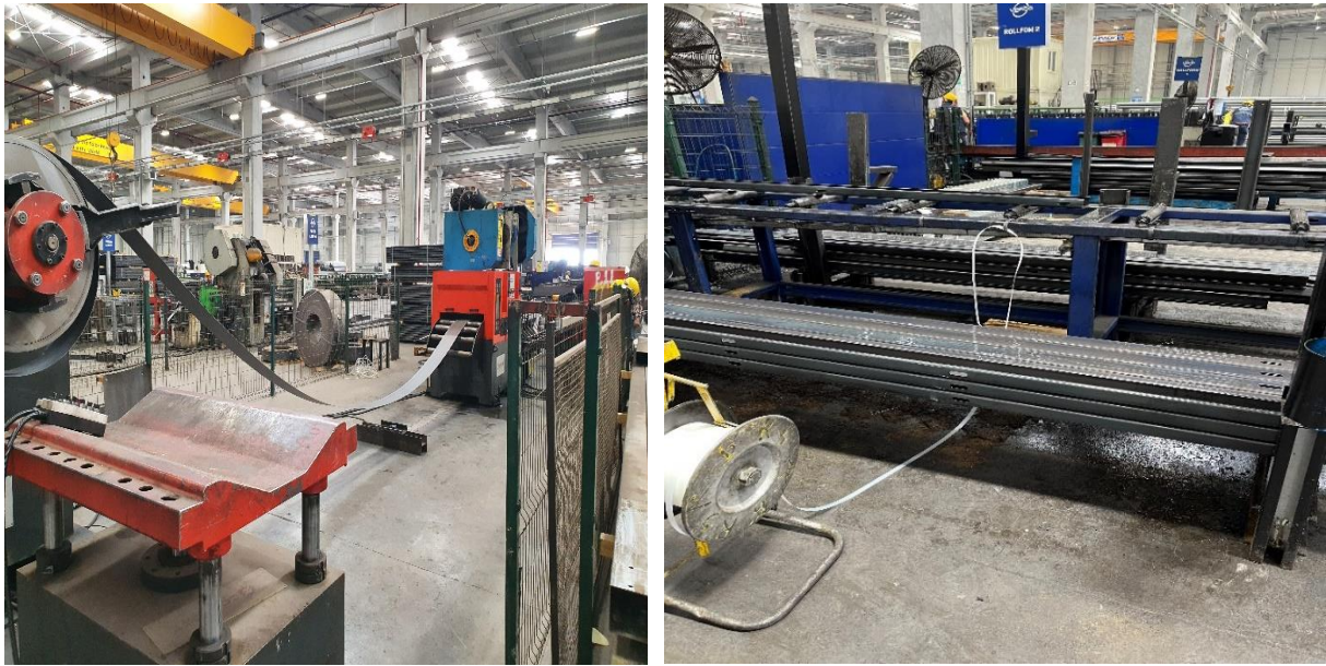
Figure 6. Press Brake and Rollform for Steel Plate Bending
